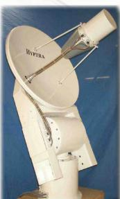
This station is designed for signals reception from 1 to 18 GHz in three sub-bands. The feed is can be equipped in option with a YIG filter for short loop tests. It is operated in Remote (RS 232C) or Local mode.
